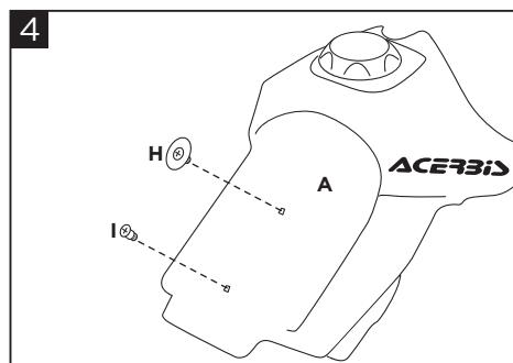
**Reassemble the seat fixing screw (H) and elastic hook fixing screw (I) on the Acerbis fuel tank (A).**
