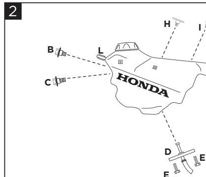
**Remove the bracket (L) from the original tank through the screws (B) and (C), the connector (D) through the two screws (E) and finally the seat fixing screw (H) and elastic hook fixing screw (I).**
