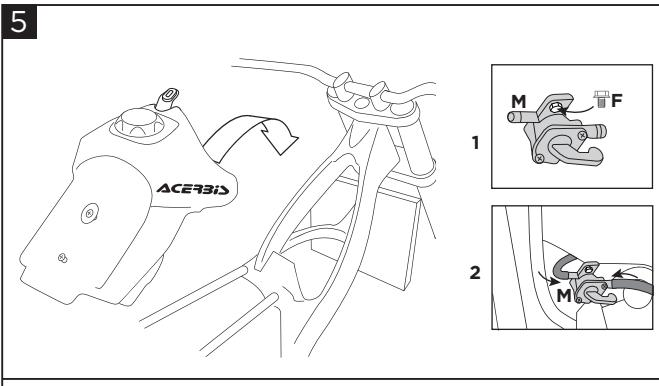
**Mount the tap (M) using the screw (F) on the Acerbis fuel tank (A) and place it on the bike.**
