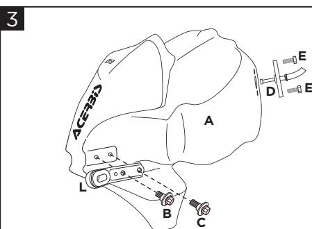
**Reassemble the bracket (L) on the Acerbis fuel tank (A) using the screws (B) and (C) and the connector (D) using the two screws (E).**
