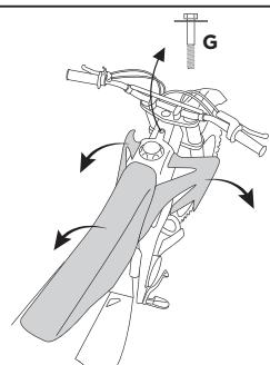
**Remove the seat and the radiator side panels. Unscrew the screw and washer (G), release the original elastic, disconnect the petrol pipes and remove the tank. Unscrew the screw (F) and remove the original tap (M).**
