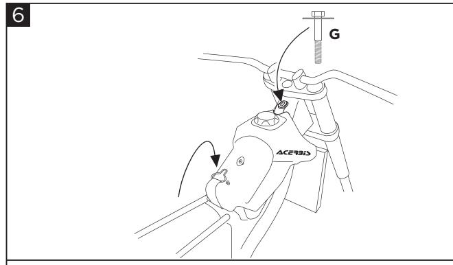
**Fix the tank using the original elastic band and block it using the screw and washer (G) in the bracket (L). Finally insert the petrol pipes.**
